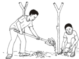
3. Fill each hole with sand and stone to pack the sticks tightly so that they don't move
