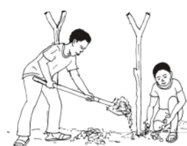
3. Fill each hole with sand and stone to pack the sticks tightly so that they don't move
