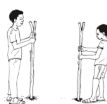
2. Place one forked stick in each hole. Make sure they are the same height
